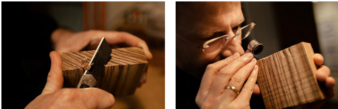
Fig. 1. Preparation of the transverse plane and macroscopic observation / identification of the timber
